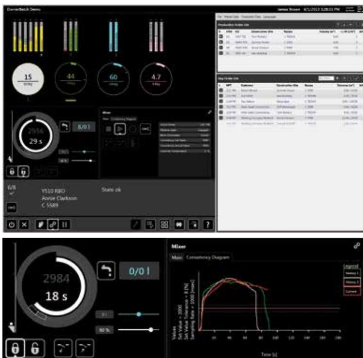
SIMEM@TIC 3.0 is the automation program that, with a friendly interface, displays all the essential information about the plant for full operations control (loading, weighing, recipes, discharge, production lists, pending orders,...)
